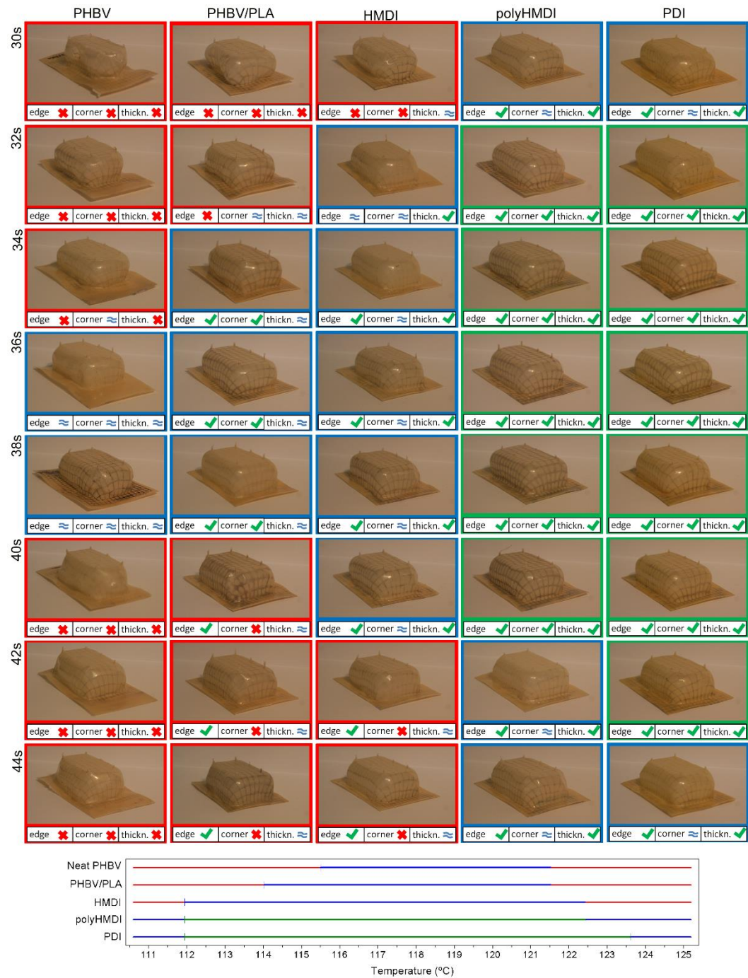
Fig. 6.6: Photographs of the thermoformed structures depending on the processing temperature and thermoforming temperature range for Neat PHBV, PHBV/PLA blend and the PHBV/PLA compatibilized blends.
