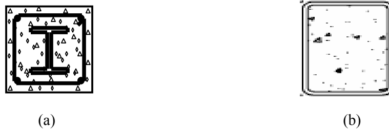
Figure 6. Types of Composite Column (a) Encased Column (b) Concrete Filled Tubular Column
