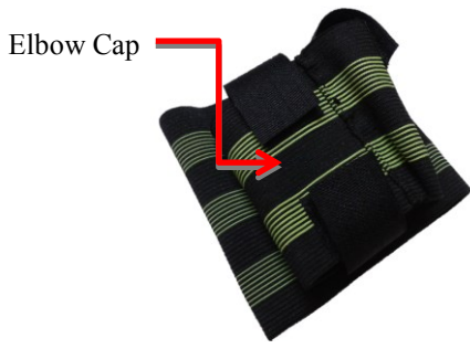
Figure 4. The developed pouch bag for sensor housing.
