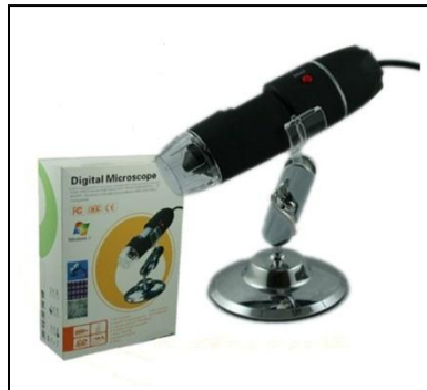
Fig. 4: Digital microscope used for particle shape quantification
