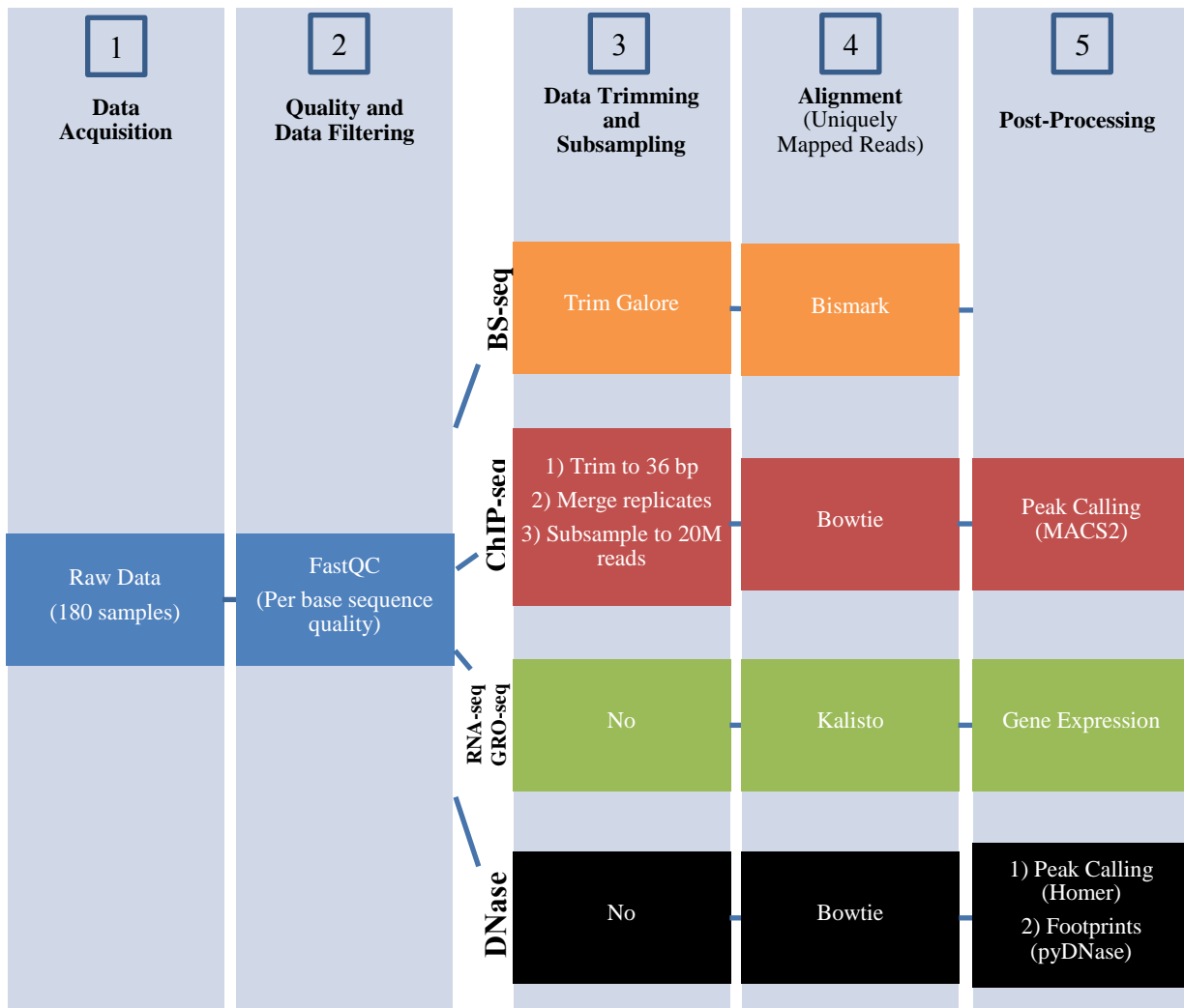
Figure 2.1 – Analysis pipeline according to each type of dataset from NIH Roadmap Epigenomics Data.
