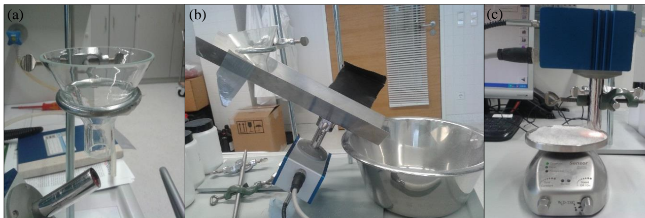
Figure 6: Experimental setup for off-line NIR spectra acquisition: (a) Funnel experiment, (b) Chute experiment, (c) Rotating plate experiment.
