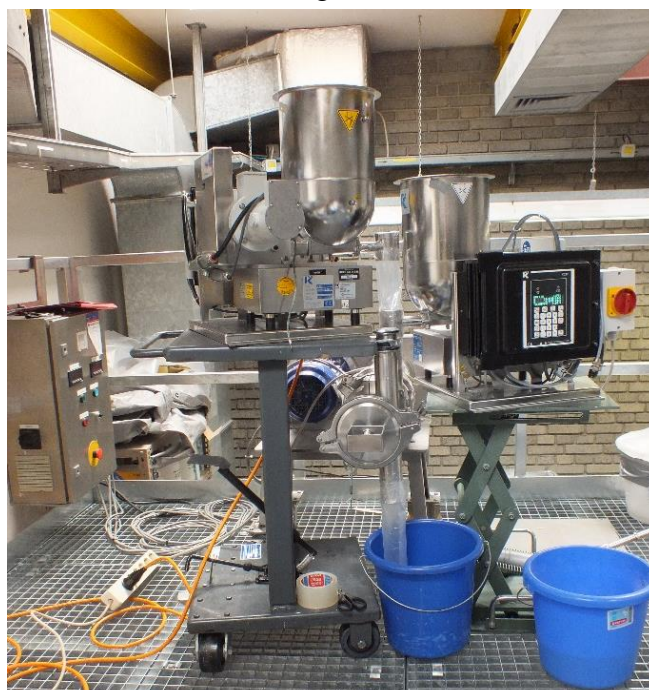
Figure 19: Experimental setup for continuous blending study.
