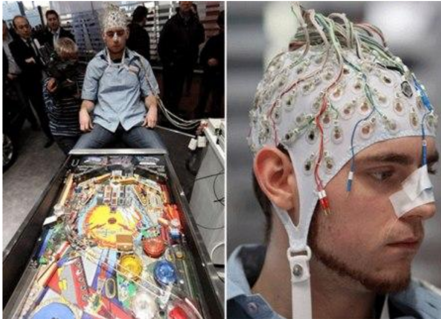
Figure 3.1: BCI game pinball from (Krauledat et al., 2009) demonstrated in the CeBIT exhibit in Hanover, Germany (2010). Here, each flipper of the arcade game was activated by using a sensorimotor activity approach.
