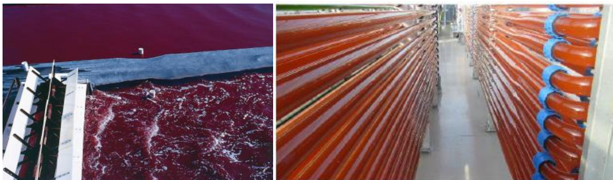
Figure 1.8 – Two examples of cultivation systems used at industrial scale. Culture ponds (500 000 liters) at Cyanotech Corporation (HI, USA) (left image); H. pluvialis production in photobioreactor at A4F (right image).
