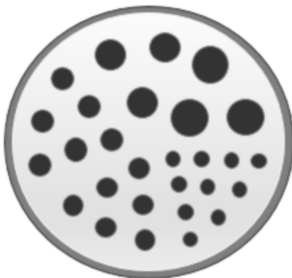
Figure 3.7: Draw of the Simulated Derenzo phantom for small animal PET. Derenzo phantom composed by rods with radius of 1.2 mm, 1 mm, 0.75 mm, 0.675 mm and 0.5 mm.
