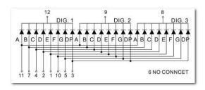
having 11 conductors, we can control 24 LEDs of the indicator.
