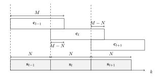
Fig. 2. Illustration of the interference pattern between consecutive blocks.
