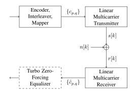
Fig. 3. Multicarrier system block diagram.
