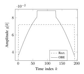
Fig. 5. Time domain representation of rectangular and out-of-band energy (OBE) minimization pulse shaping filters.
