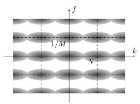
Fig. 1. Representation of the transmitted signal in the time-frequency plane.
