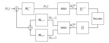
Fig. 4. Block diagram of the zero-forcing turbo equalizer.
