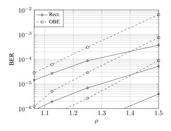
Fig. 8. BER performance as a function of  $\rho$  after 3 iterations for  $E_b/N_0 = 6, 7, 8$  dB (from top to bottom), N = 128 and K = 2048.
