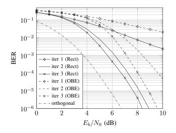
Fig. 6. BER performance as a function of  $E_b/N_0$  with  $M = 192, N = 128, \rho = 1.5$  and K = 2048.
