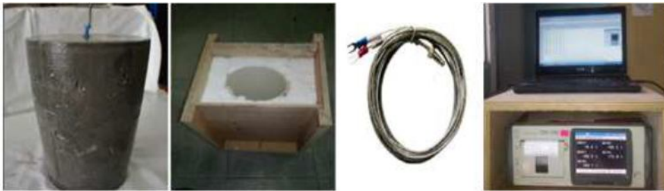
Figure 2: Test set up for the measurement of heat of hydration
