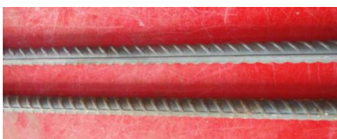
Figure 2: Deformed steel bar
