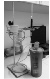
Fig. 2 Retort stands with thermo recorder and hot wire anemometer
