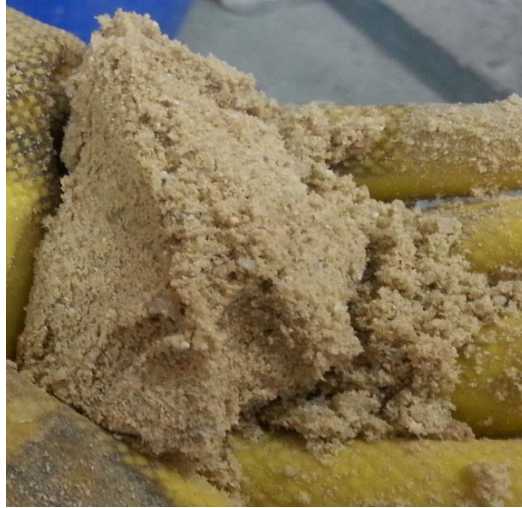
Figure 1: Fine aggregate in saturated surface dry condition
