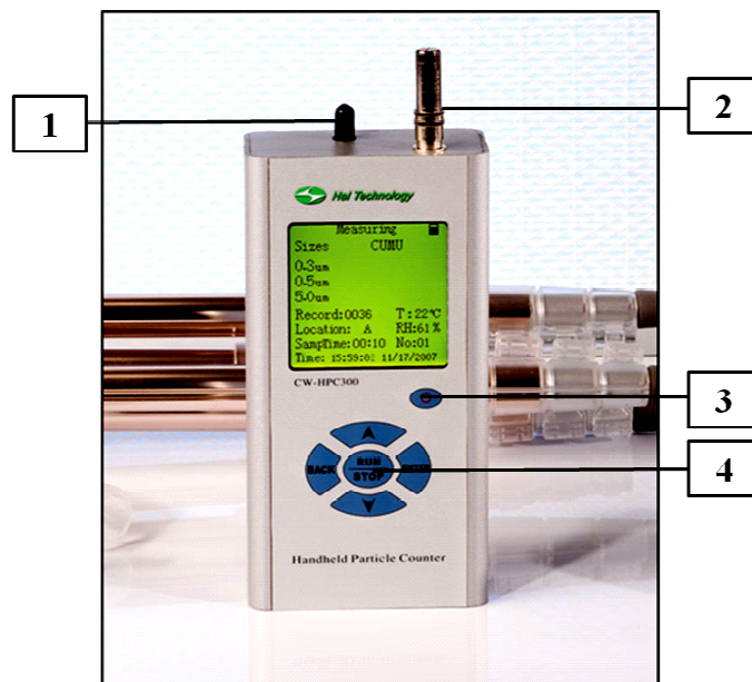
NB: 1. Air intake; 2. Temperature and relative humidity probe; 3. Power switch; 4. Control panel
