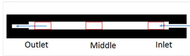
Figure 2.12: Different positions for the gray values measurements along the microchannel, when dark zones were formed.
