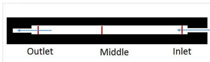
Figure 2.11: Different positions for the gray values measurements along the microchannel.
