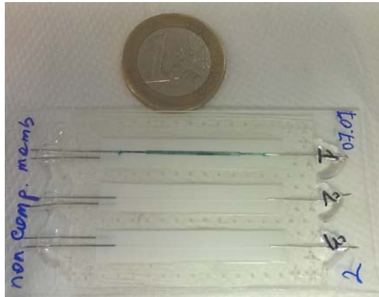
Figure 3.1: Photo of MMD after filtration of solution of dye in one of the microchannels.
