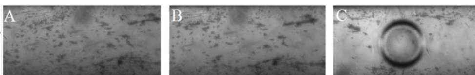
Figure 4.15: The state of membrane surface before (image A, time point 5100 s) and after (image B, time point 5400 s) the passage of air bubble captured in image C. Magnification: x50.
