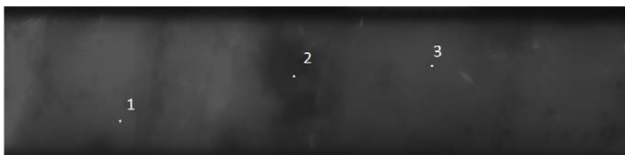
Figure 3.9: The appearance of the membrane surface at perfect focus after fouling with fluorescent BSA. (Positions 1, 2 and 3 are arbitrary selected at regions with visually different fluorescent intensity). Magnification: x50.
