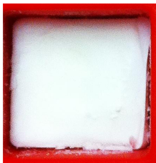
Fig. 9 Photograph of CSM containing CDDP NPs. Note the smooth surface texture and pure white color. 1.5 cm × 1.5 cm × 2 mm.
