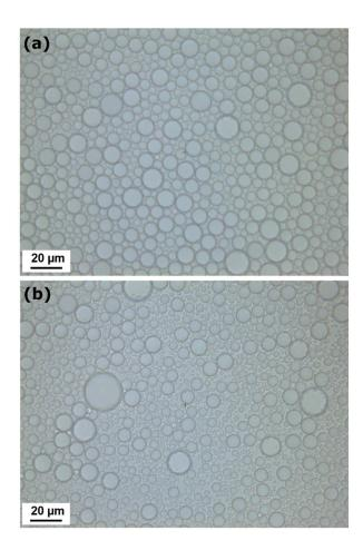
**Figure 1.** Representative emulsion photomicrographs taken on as-made (top) emulsion and 4 hr after preparation (bottom). Using 10 photomicrographs at each time, the mean droplet diameter was observed to decrease from an ensemble-averaged value of  $8.4\pm3.8~\mu m$  to  $5.8\pm3.4~\mu m$  after 4 hr. Thus, the emulsions are sufficiently stable to perform hydrate formation experiments by extended cooling.
