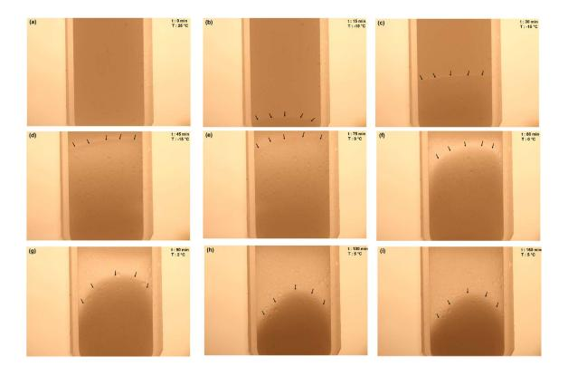
**Figure 2.** Pictures of cyclopentane hydrate formation from a 17:1 (mole ratio) water:cyclopentane emulsion inside a glass cuvette were taken during visual observation by camera. Arrows indicate the interface of the solid and the emulsion. Video of hydrate formation can be accessed in the Supporting Information. The cross section of the cuvette is 1 cm  $\times$  1 cm.
