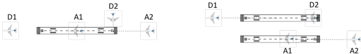
Figure 3-8. Sequence of alternating arrivals and departures on a single runway and on CSRR.
