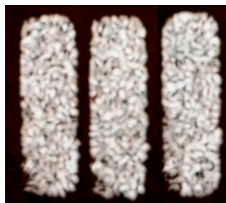
Figure 7. Three realization of modal structure in the 34x106 \mu\text{m} rectangular fiber, illuminated by a HeNe laser (that is not properly coupled to fill the fiber NA).
