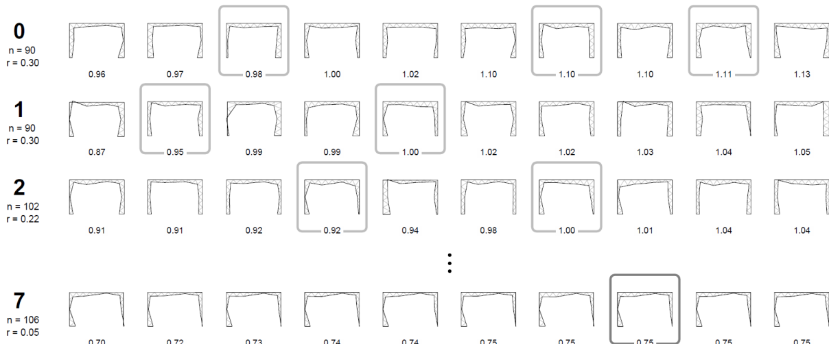
Fig. 22. Excerpt of eight successive generations for a hybrid exploration approach, in which designs are selected by the user based on both quantitative and qualitative performance.
