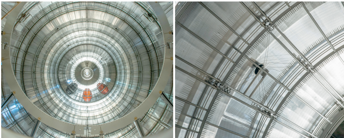
Figure 4. Left: view of the complete wire-electrode system as seen from the beam-line flange at the source end of the MS. At the far end the three pump ports with the LN 2 baffles are visible. Right: voltage distribution to the corners of an electrode module from the distribution panel underneath a flange with electrical feedthroughs.
