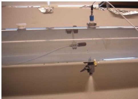
(a) Hydrophone and DPT during opened leak experiment
