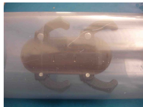
FIGURE 14. The mobility module prototype inside a 100mm pipe section. The module is stable due to the support provided by the legs.
