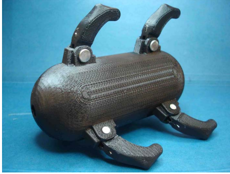
FIGURE 4. Our first prototype. ABS plastic along with a 3D printer was used for prototyping.
