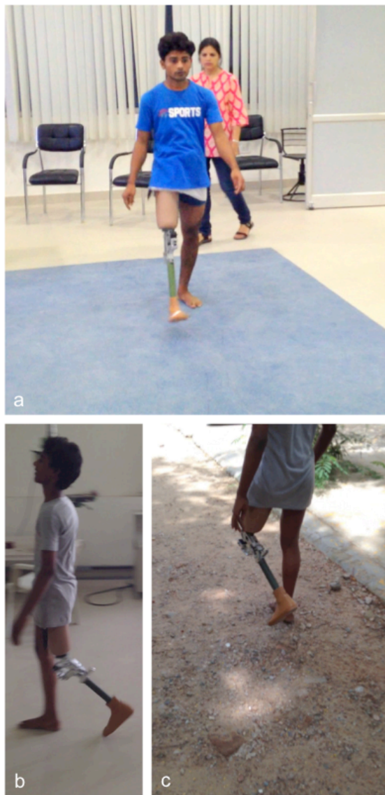
Figure 4. PRELIMINARY FIELD EVALUATION. Fig. 4a. Subject 1 using the prototype for the 2-minute walk test. Fig. 4b. Subject 2 during the 2-minute walk test, late stance flexion of up to 40 degrees can be seen. Fig. 4c. Subject 2 walking outdoors on uneven terrain.
