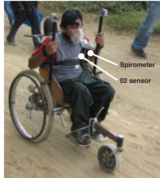
FIGURE 2. LFC trial subject in Guatemala wearing biomechanical testing equipment. The mask worn by the subject is connected to a spirometer and oxygen sensor, which measure oxygen consumption rate (VO 2 ).
