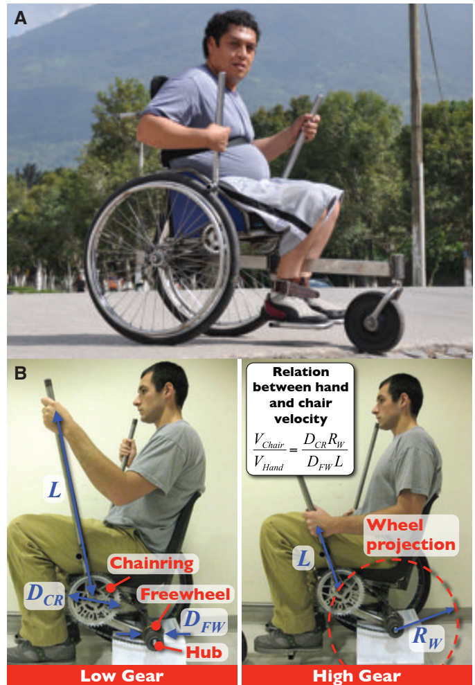
FIGURE 1. The Leveraged Freedom Chair (LFC). A) Perspective view of a Guatemalan trial subject in the LFC. B) LFC variable mechanical advantage, single speed drivetrain. All components in the drivetrain are made from bicycle parts found anywhere in the developing world. Inset gives the mathematical relationship for how the ratio between LFC speed ( V_{Chair} ) and pushing speed on the levers ( V_{Hand} ) varies as a function of the effective lever length ( L ), which is determined by hand position on the levers. Other labels: diameter of the chainring ( D_{CR} ), diameter of the freewheel ( D_{FW} ), and rear wheel radius ( R_W ).
