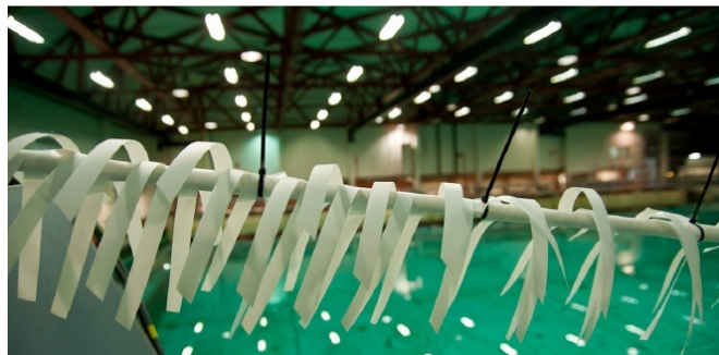
Figure 1. Pipe 1 covered with ribbon fairings
