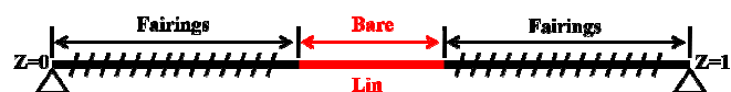
Figure 5. Schematic of Pipe 1 with fairings at two ends of the pipe, leaving a gap (bare region) in the centre
