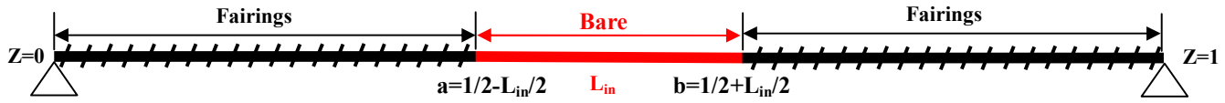
Fig.1: Configuration of the pipe with fairings. The exposed region (Bare region) was always in the middle of the pipe and the fairings were installed symmetrically towards both ends of the pipe.
