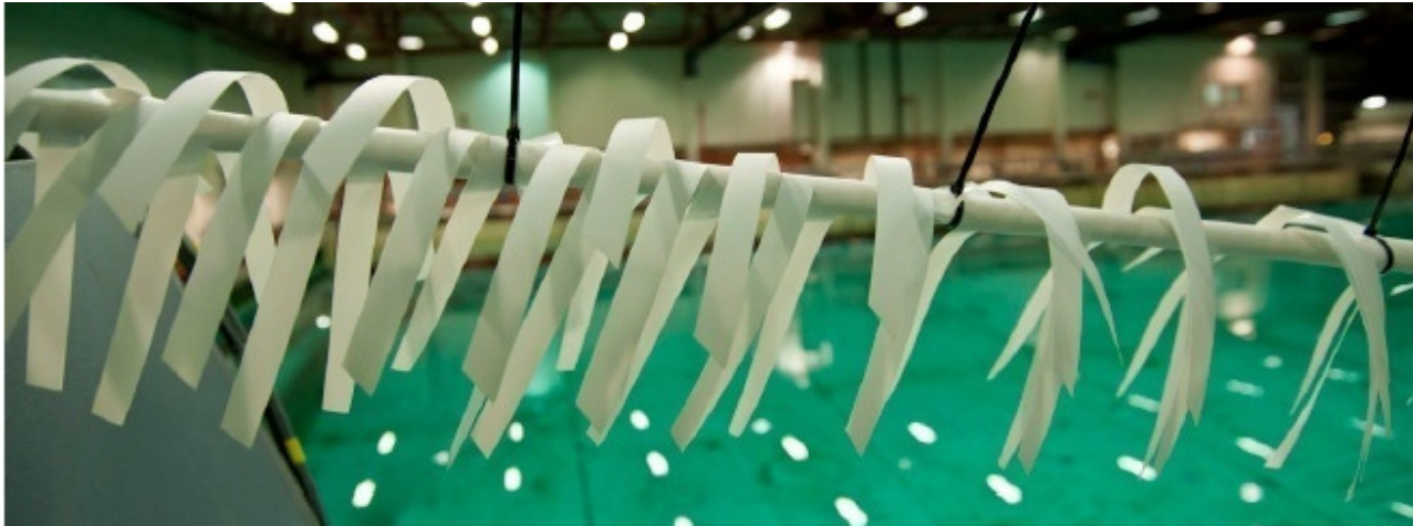
Figure 2: Small pipe covered with wrapping ribbon fairings
