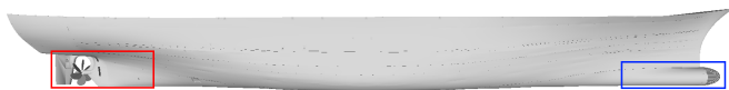
Fig. 7. Inspected regions of the hull of the SS Curtiss for the running gear (red) and bulbous bow (blue) datasets.
