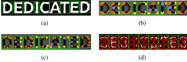
Fig. 4. Word encoding with junction features: (a) Binarization of the original image overlaid by detected regions (green rectangles), (b) visualization of junction binary patterns (JBPs), colored by number of line segments (1: yellow, 2: orange, 3: blue), (c) junction keypoints aggregated from (b), and (d) a visualization of JBP by 2x3 grids in each region.
