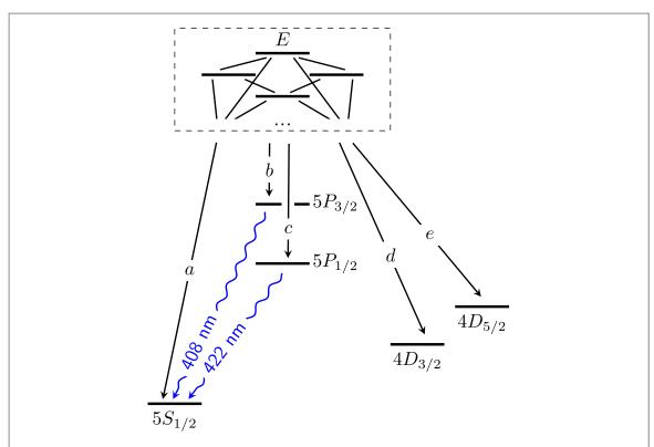
**Figure A1.** The base branching ratios of an arbitrary state E in <sup>88</sup>Sr<sup>+</sup>, effectively the branching ratios of the set of states consisting of E and all states higher than the five lowermost states that E decays to. Only detecting 422 and 408 nm photons from various population transfers is sufficient for measuring base branching ratios.
