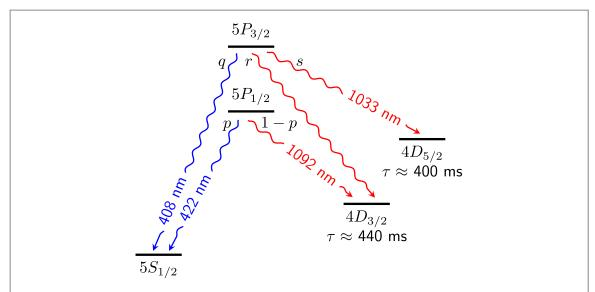
**Figure 1.** Energy levels of  $^{88}$ Sr $^+$ , showing the  $5P_{1/2}$  and  $5P_{3/2}$  excited states and their decay channels.  $4D_{3/2}$  and  $4D_{5/2}$  are metastable states with lifetimes much greater than the timescale of the experiment [26]. To measure the  $5P_{3/2}$  branching ratio, we need only lasers addressing the 408, 422, 1092, and 1033 nm transitions.
