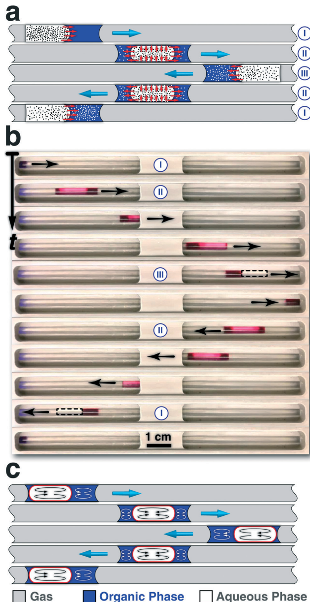
Fig. 3 (a) Microscale mixing of two immiscible fluids using oscillatory multiphase flow strategy for in situ studies of intra-phase transport processes. (b) Snapshot time-series of the oscillatory motion of a bi-phasic slug (clear phase: DI water, 15 \mu L, red phase: 1-octanol labelled with Sudan red, 10 \mu L, gas: pressurized nitrogen) in a tubular FEP reactor, during one complete oscillation cycle. (c) Ideal microscale mixing of two immiscible fluids using oscillatory multiphase flow strategy for in-flow studies of bi-phasic interfacial catalytic reactions. The available interfacial area for the multiphase process is highlighted in red. Adopted with permission from the American Chemical Society, 2015 (b). 69
