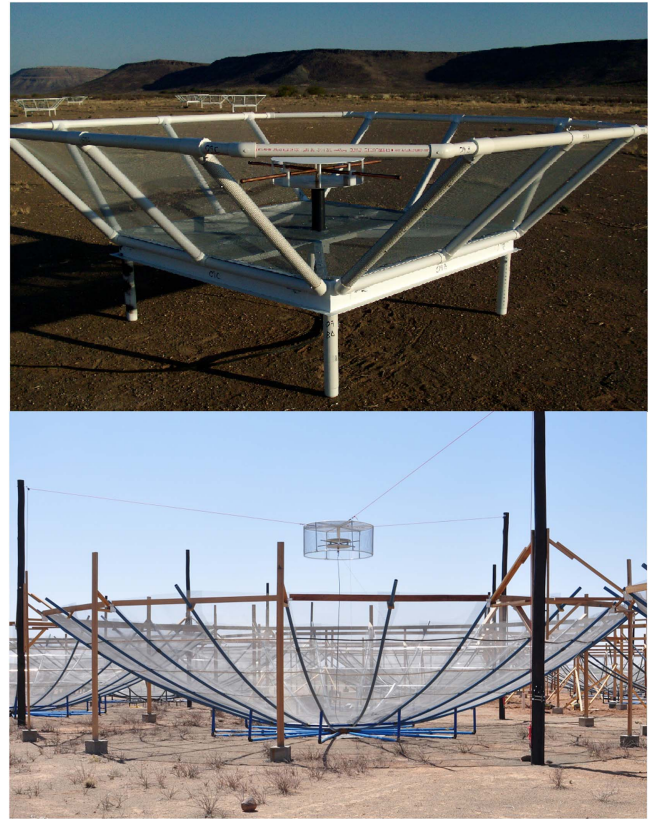
Figure 1. HERA antenna element (bottom) uses a parabolic dish to achieve an order of magnitude increase in collecting area over the PAPER antenna (top). The sleeved dipole in the center of the PAPER backplane is identical to the sleeved dipole being suspended under the cylindrical skirt over the vertex of the HERA dish. The suspended feed arrangement has the potential to introduce intra-antenna reflections, which we explore in this work.
