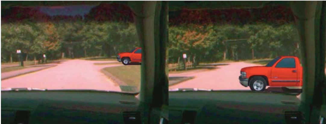
Figure 2. Two images of a video showing superimposition of computerized truck images on an actual driver's view in a test drive on a country road. White objects are fiducial markers to enable continuous geometric correspondence of the AR image to the real world.
