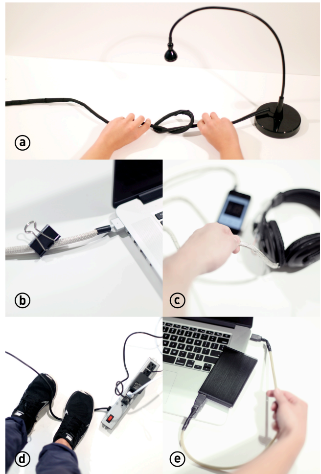
Figure 2: The five prototypes. a) embedded bend sensor detects knot's tightness. b) we can sense the clamp's pressure using conductive polymer. c) conductive yarn woven into the cord sleeve senses touch and pressure. d) special piezo copolymer cable can detect kinks. e) stretchable cord with rubber resistive cord to sense pulling.
