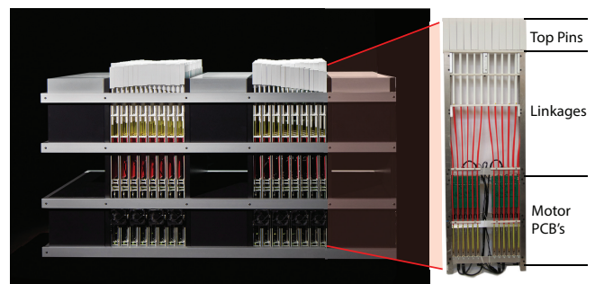
Figure 13. Side view of the TRANSFORM system with a single 12x2 actuation module.
