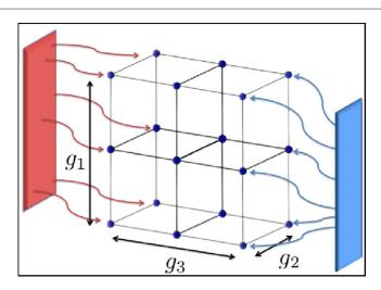
**Figure 1.** Sketch of a d=3 lattice with  $L_1=3$ ,  $L_2=2$ , and  $L_3=3$ . Local thermal baths apply at the terminal sites of dimension 3.
