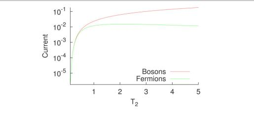
**Figure 2.** Energy current (logarithmic scale) for a fermionic and bosonic system as a function of the temperature of the hot bath.  $\Gamma_1 = \Gamma_2 = 0.01, \ \ \omega = 10, \ T_1 = 0.001, \ d = 1.$
