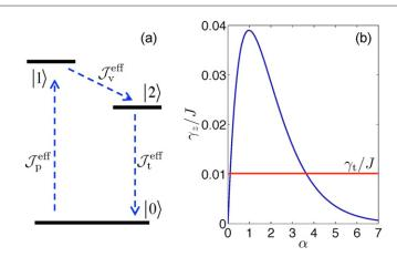
**Figure 5.** (a) The kinetic model of a single excitation transfer cycle. In the strong coupling regime, the energy transfer processes between different local states can be described by the effective fluxes. (b) The relaxation rate  $\gamma_z$  versus system—bath coupling strength  $\alpha$ . The red line indicates the trapping rate  $\gamma_t$ . The parameters here are the same with figure 3.
