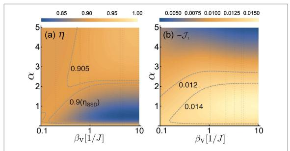
**Figure 7.** The dependence of (a) the energy transfer efficiency and (b) the trapping energy flux on the coupling strength and temperature of the phonon bath. The temperatures and dissipation coefficients of the pumping and trapping bath are the same as in the figure 4.
