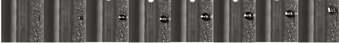
Fig. 3. Consecutive images of a bubble from its initial growth to its departure.
