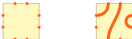
Fig. 1. Square tile with two vertices per side and non-intersecting paths between them.
