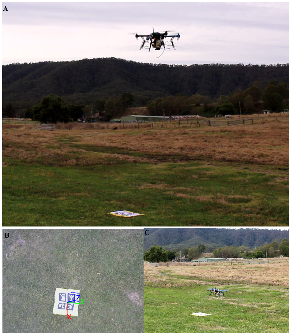
Figure 6.2: A: The marker target is detected. B: Detecting target. C: Hovering above the target after detection.
