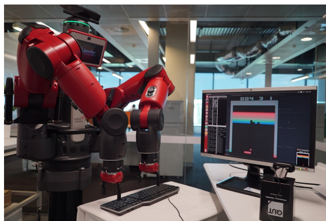
Figure 1: Three different game screen environments were used across the training and testing of both agent DQN[1] and our agent. 1a is an example of the pristine game screen images used in [Mnih et al. , 2015]. 1b is an example of the game screen images used to train our agent. 1c is an example of the noise caused by viewing the game screen through a low cost webcam. 1d shows the Baxter robot playing Atari 2600 game Breakout through a webcam’s view of the game screen.
