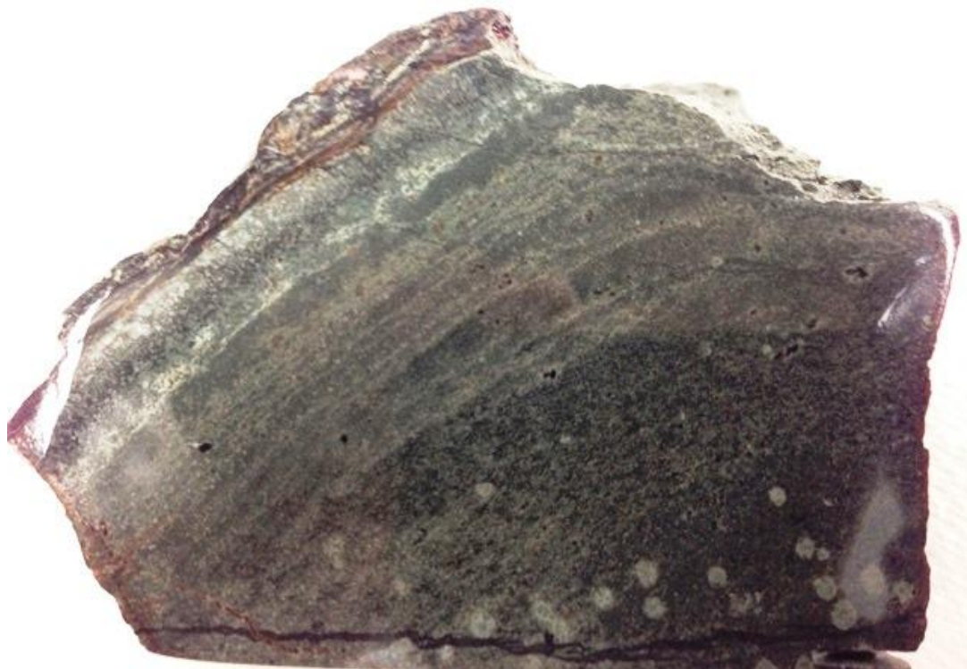
Figure 17. Image of cut surface of sample TS-37-1-14. The image shows the quenched rim of the pillowed basalt as well as evidence of possible multiple flows and disseminated ocelli (2 to 5 mm).
