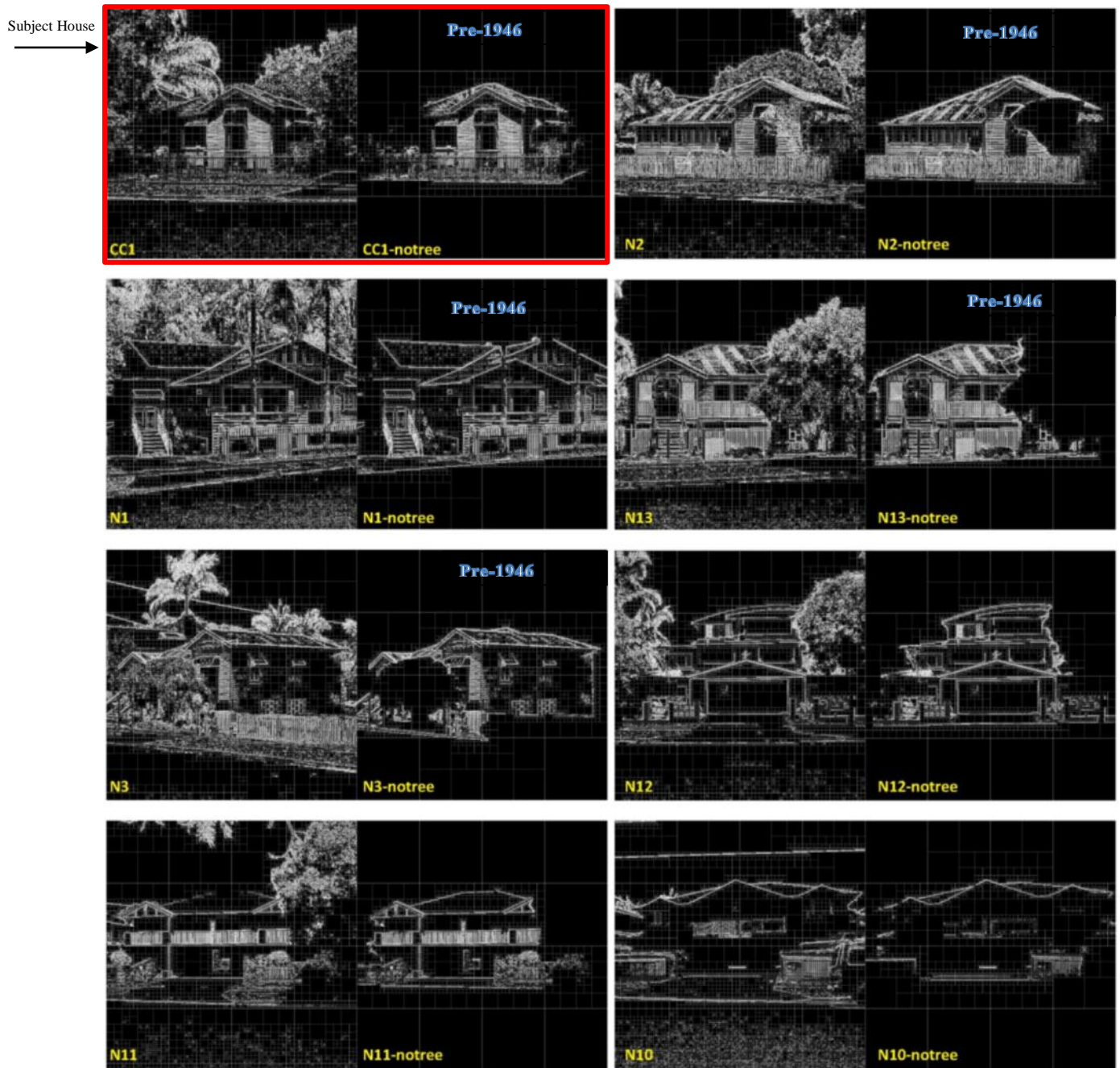
Figure 5-14. Transformed Collins Street Photos by Quadtree Decomposition (with and without vegetation options)
