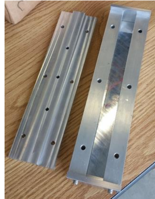
Aluminum mold used to cast the samples
