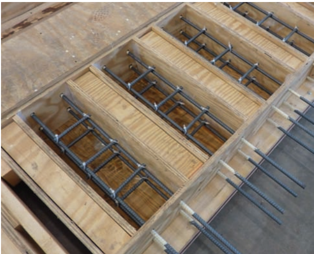
Figure 4.17 Example of black bar specimens ready for casting.
