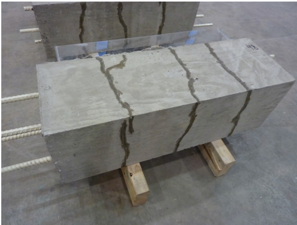
Figure 4.34 Typical specimen with cracks sealed on sides and bottom with silicone.
