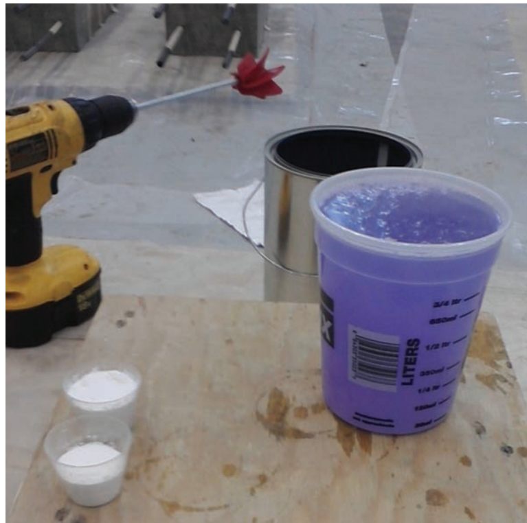
Figure 4.29 Measured quantities of component materials for Degadeck Crack Sealer Plus.
