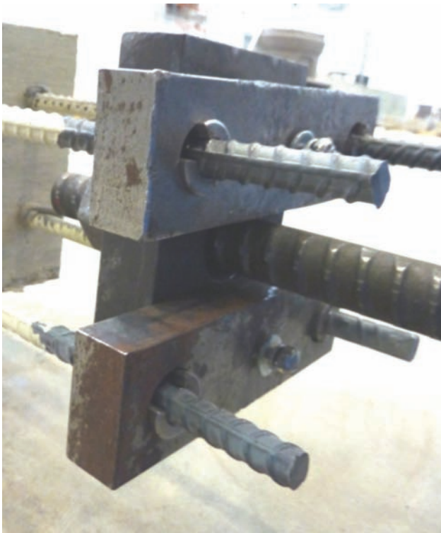
Figure 4.23 Wedges connecting reinforcing steel to transfer plates.
