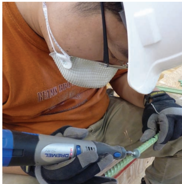
Figure 4.4 Introducing damage to epoxy-coated bar.
