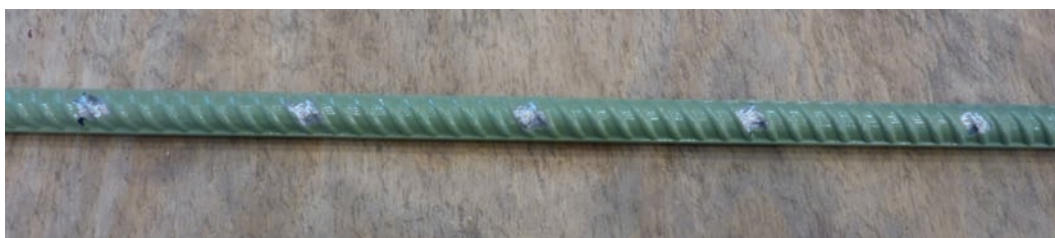
Figure 4.5 1/4 x 1/4 in. damage areas on longitudinal bar.
