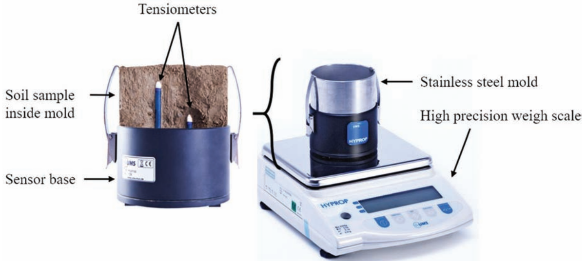
Figure 2.10 Decagon HYPROP device for tensiometer measurements.
