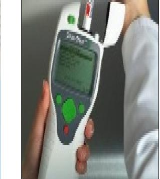
Expose the experimental sample to the luciferase containing swab & reinsert the swab in the swab tube. Measure the florescence efficacy in ATP illuminometer
