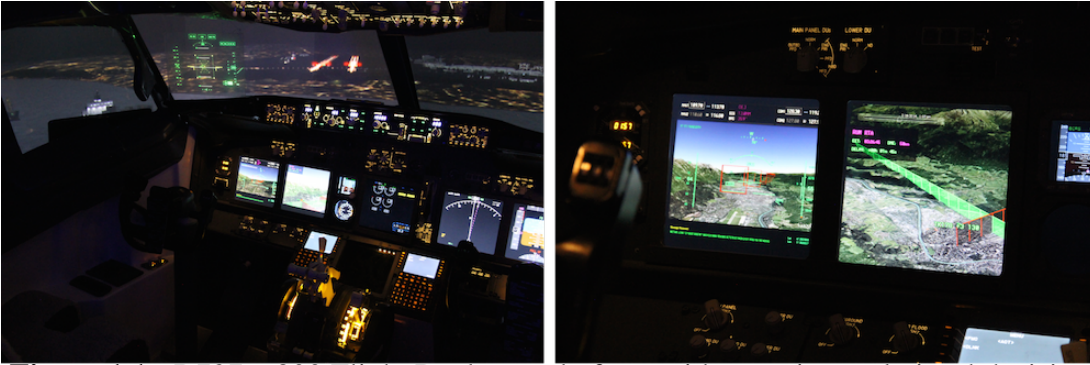
Figure 1.1 : B737 – 800 Flight Deck test platform with experimental visual decision support tools for future ATM realm: Head up Display (HUD), Synthetic Vision Display (SVD) and 4D Operational Display
