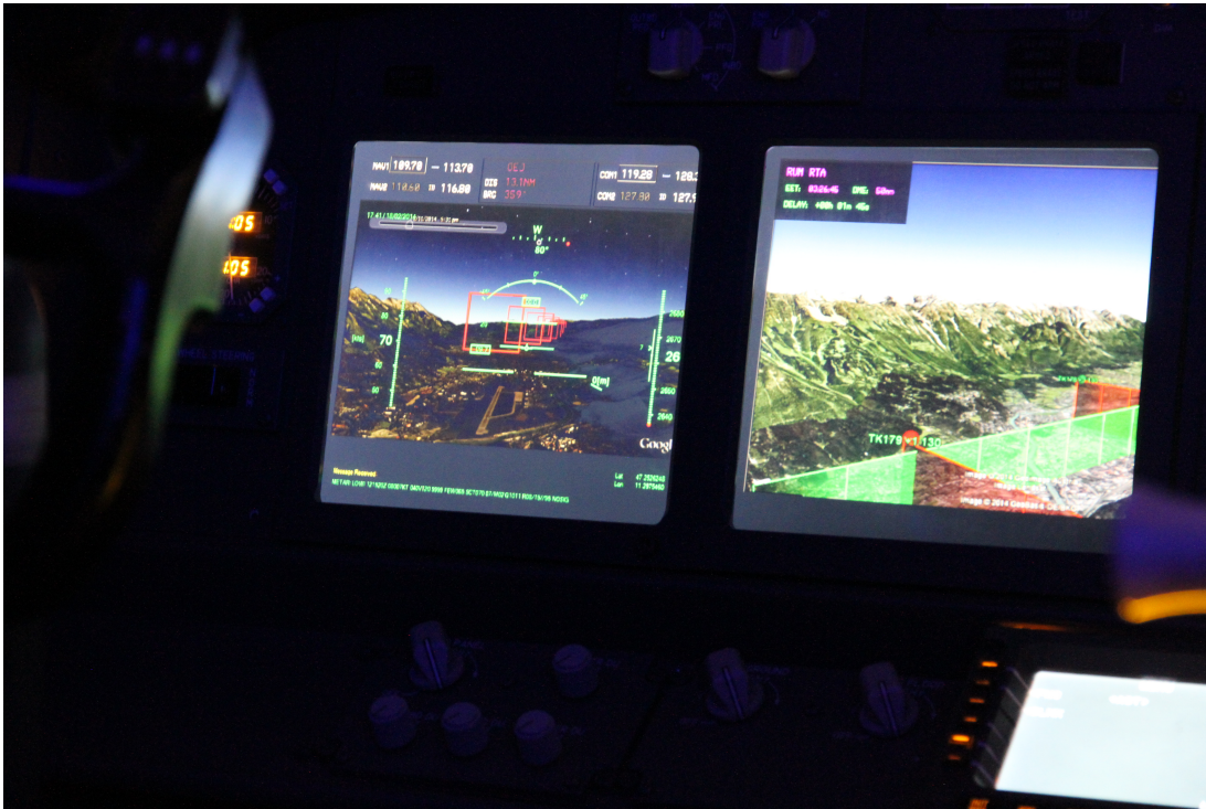
Figure 2.4 : Synthetic Vision Display (SVD) and 4D Operational Display (4DOD) screens in the flight deck
